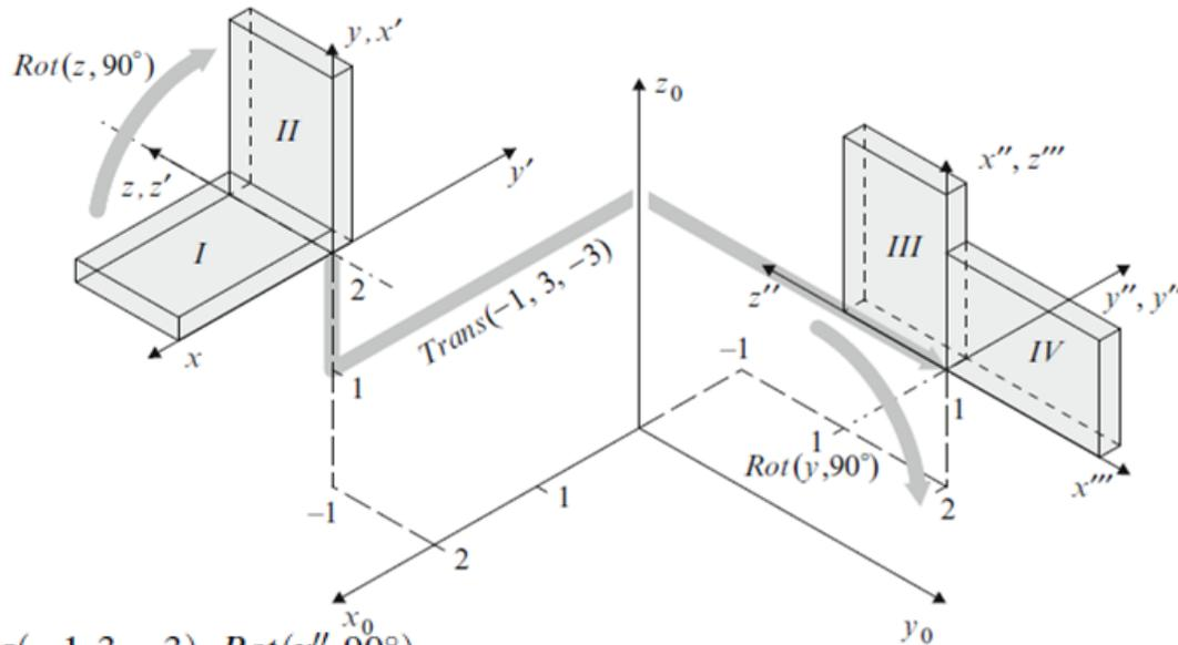
$$\mathbf{D} = \text{Rot}(z, 90^\circ) \cdot \text{Trans}(-1, 3, -3) \cdot \text{Rot}(y', 90^\circ)$$
