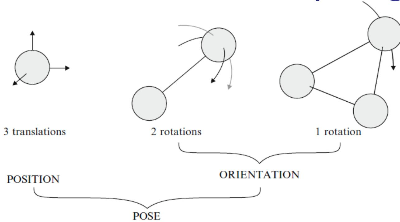
A single mass particle has three degrees of freedom, described by three rectangular displacements along a line called translations (T).
