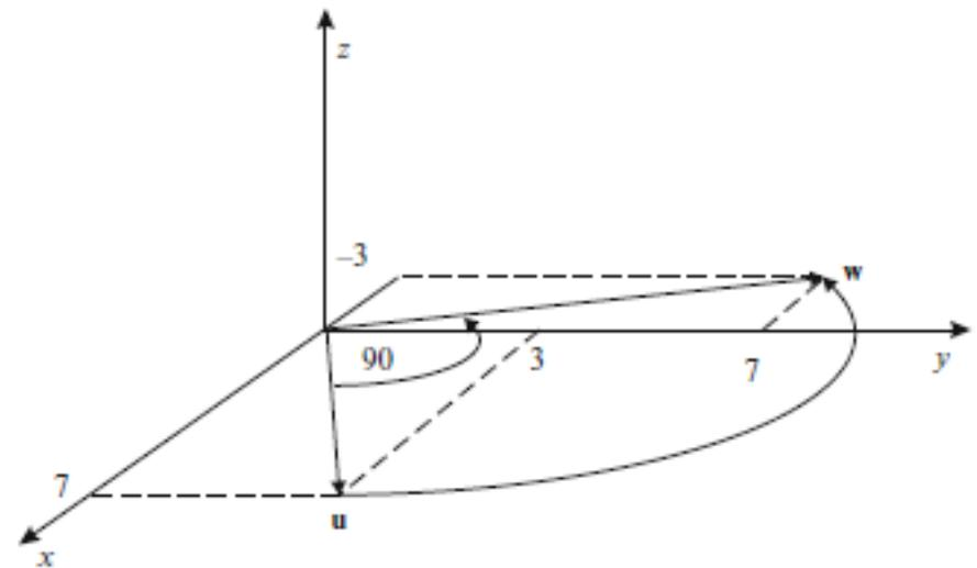
$$Rot(z, \gamma) = \begin{bmatrix} \cos \gamma & -\sin \gamma & 0 & 0 \\ \sin \gamma & \cos \gamma & 0 & 0 \\ 0 & 0 & 1 & 0 \\ 0 & 0 & 0 & 1 \end{bmatrix}$$
