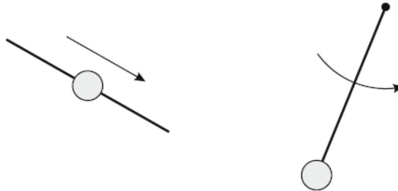
Fig. 1.1 Two examples of systems with one degree of freedom: mass particle on a wire (left) and rigid pendulum in a plane (right)
