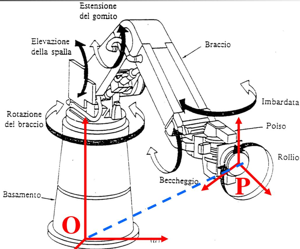
$$\mathbf{x} = (p, \Phi) = (x, y, z, \text{roll}, \text{pitch}, \text{yaw})$$
