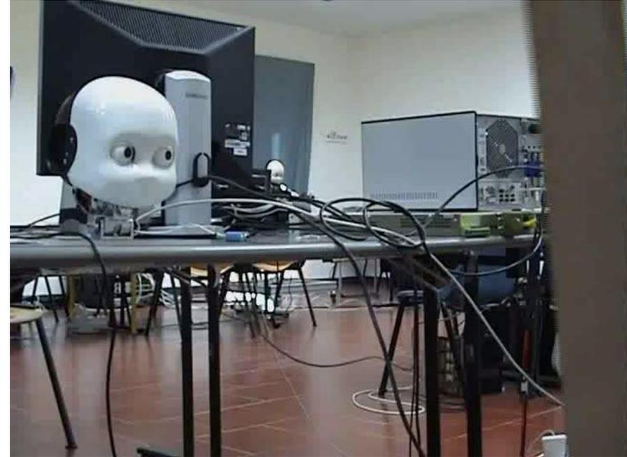
The tracking algorithm based on particle filtering detects the position of the target on the image and sends the results directly to the smooth pursuit system. When the target reappears, **the gaze points to the position of the target reappearance**, so the tracking algorithm is able to find the ball at the center of the image.
