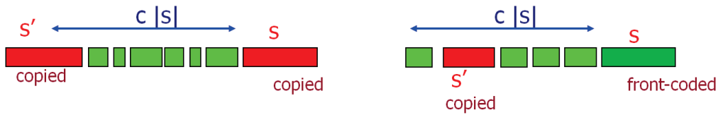
FIGURE 1.5: The two cases occurring in LPFC. Red rectangles are copied strings, green rectangles are front-coded strings.
